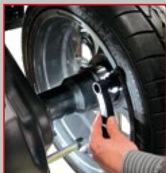
自动储存距离和直径 Automatic storage of distance and diameter.
