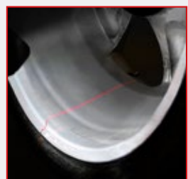
6点方向的激光线指示黏贴铅块的位置 Indicates the weight positioning with a laser line at 6 o'clock (for adhesive weights).
